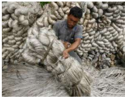
Figure 15: Final low-quality jute using traditional stem retting
